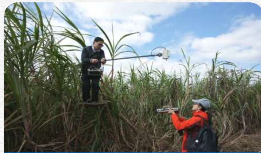
测量甘蔗光谱信息 Measuring sugarcane spectral information
